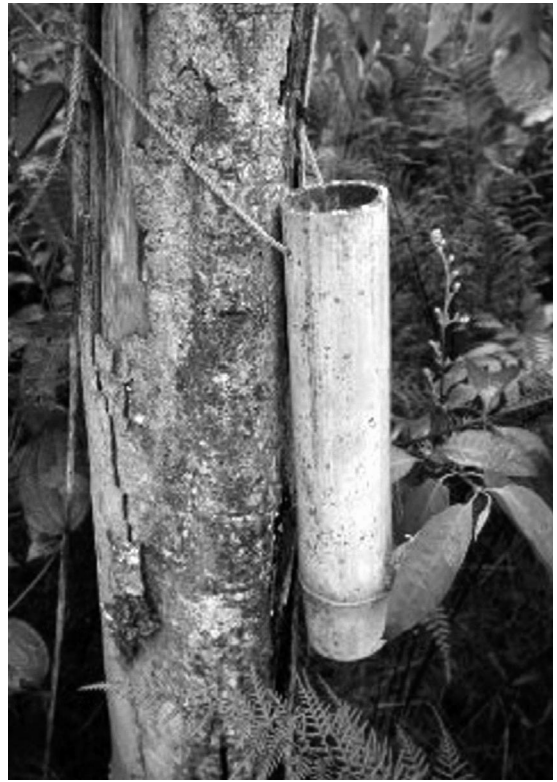
Fig. 1. Typical experimental bamboo section used in the project. The section shown is \approx 30 cm in length and has an inside diameter of \approx 6 cm.
