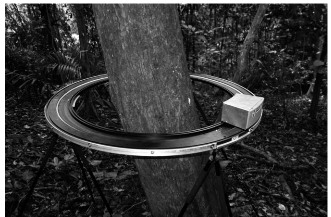
FIGURE 2. The LaserBark apparatus in place around an Anacardium excelsum tree trunk in Panama. The inside diameter of the LaserBark track is 100 cm. The small white patch on the tree trunk facing the recording unit is bait for ants.
